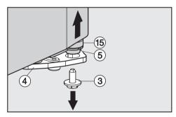
■ Unscrew retaining screw ③ on bottom right hinge plate ④.
